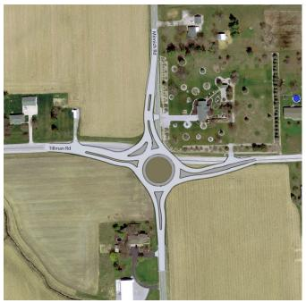
southwest of the existing intersection to minimize impact to the northeast and northwest residential properties. The project will include curb and gutter which will require a closed storm sewer system. There will also be open ditches adjacent to the project to perpetuate
